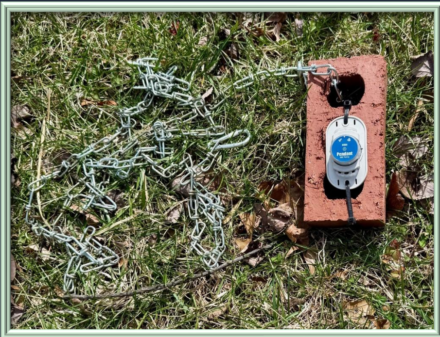
The Priority Waters team will deploy "TidbiT" model data loggers in the two project streams."
